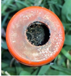
Figure 2-5. Expelled sensor with a hole drilled in top to drain liquid. Residue and bacteria growth from moisture intrusion can be seen inside the cap of the sensor. Sensors without liquid intrusion would be the same orange color inside the cap rather than the dark color.
