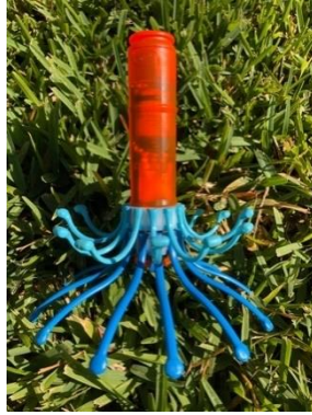
Figure 2-1. The birthing sensor from JMB North America. The orange tubular component houses the radio frequency transmitter and battery while the two blue appendages retain the sensor within the vaginal canal.
