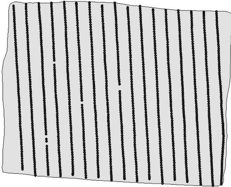
Figure 1-1. Example of  $EC_a$  data points collected by the Veris 3150 sensor cart, field 21 prior to interpolation.
