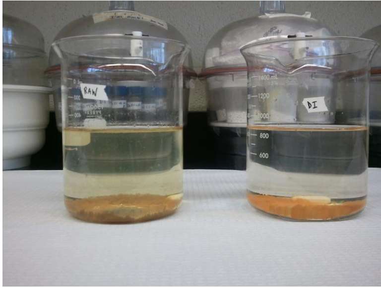
Figure A-3. Front view of PUR ® treatment of Raw and DI water for the TOC concentration test (Raw water from Lake Alice on the left, Deionized water on the right)
