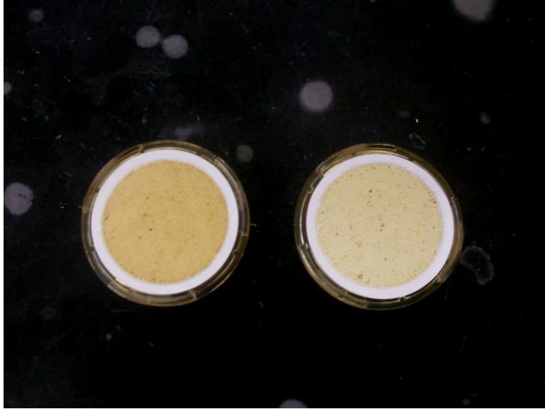
Figure A-5. Filters after vacuum filtering the Raw and DI treated water (Raw water filter is on the left, DI water filter is on the right)
