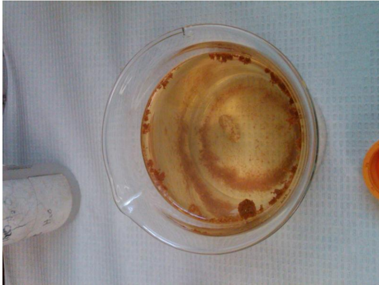
Figure A-1. Floc forming just after PUR ® mixing process
