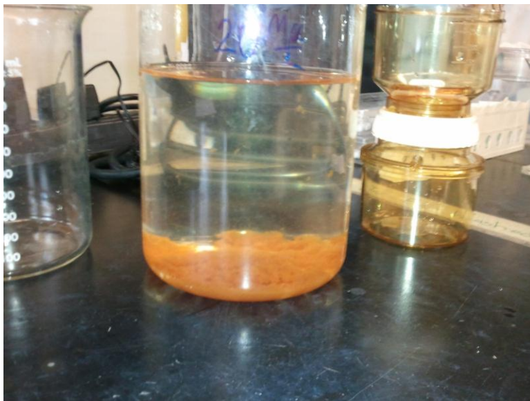
Figure A-2. Settled floc after allowing mixture to settle for the recommended 5 minute period
