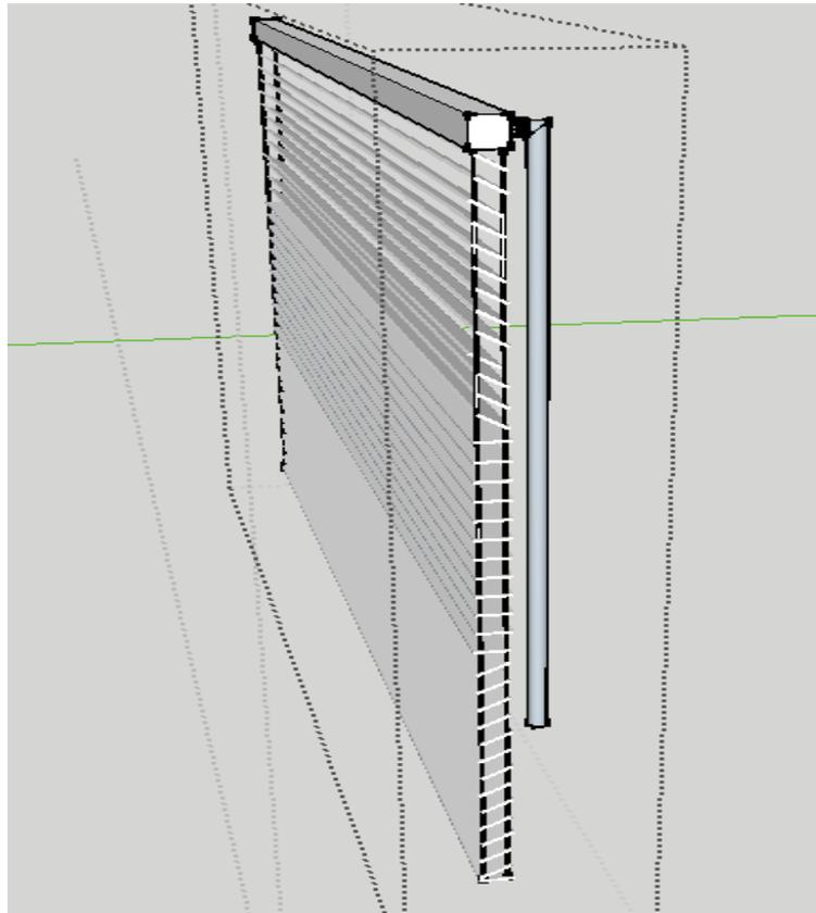
Figure 1-1. A three-dimensional view of a Google SketchUp image for the proposed split controlled blind system. The split blinds system is divided into three sections: Top section, Middle section, and Bottom section
