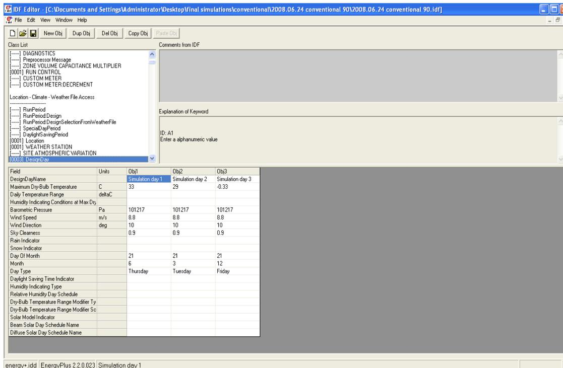
Figure 3-4. The IDF interface for Design Day Input.
