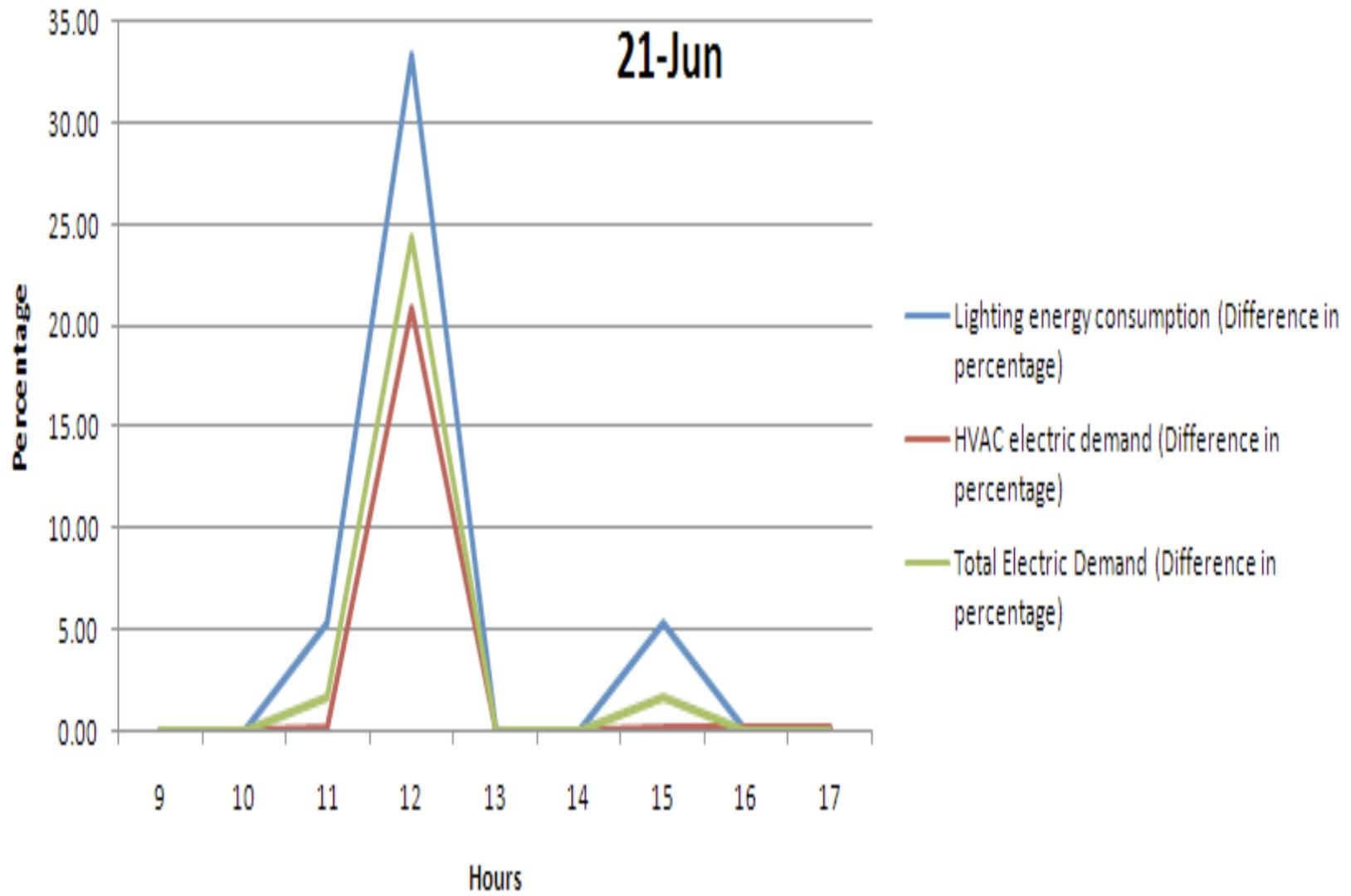
Figure 4-2. Energy consumption differences between split-controlled blinds and conventional blinds for June 21st.
