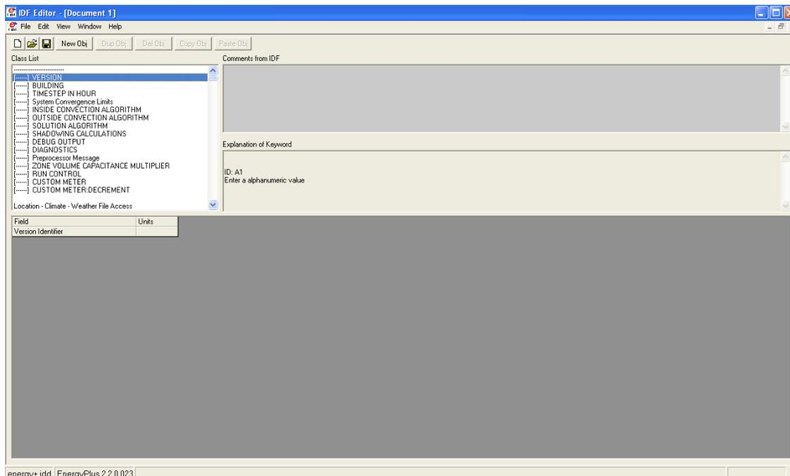
Figure 3-3. The input for EnergyPlus was done through the IDF-Editor interface.
