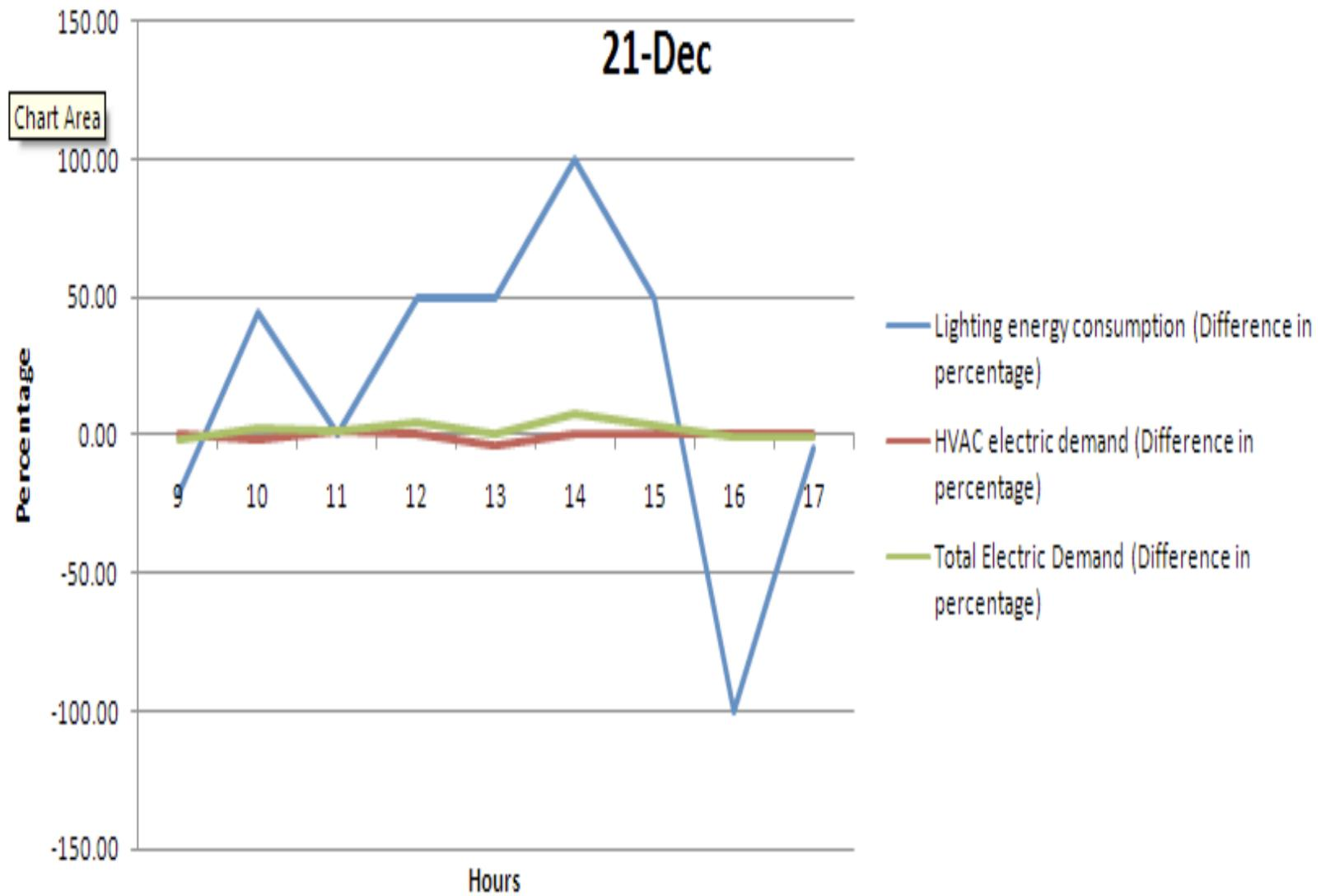
Figure 4-3. Energy consumption differences between split-controlled blinds and conventional blinds for December 21
