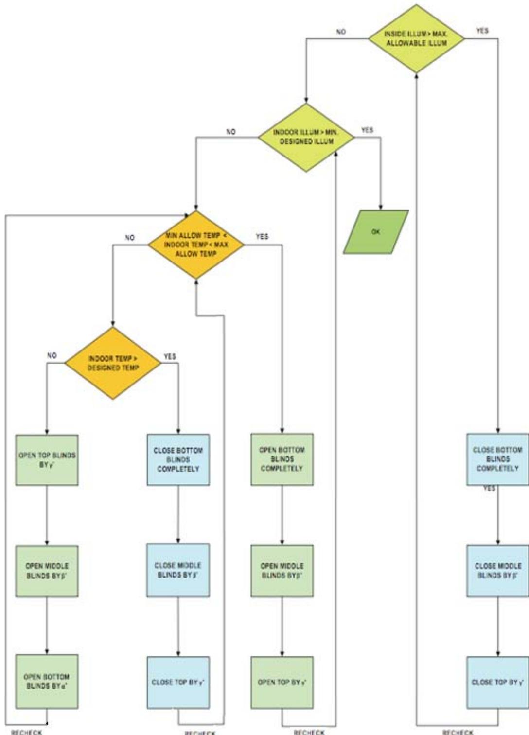
Figure 4-16. Automation algorithm for split-controlled blinds.
