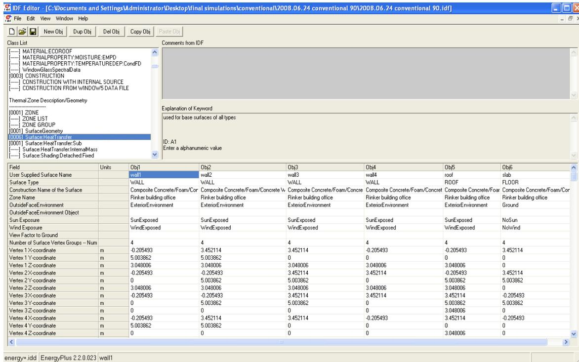
Figure 3-5. Screen shot showing all the necessary variables for the object surface heat transfer.
