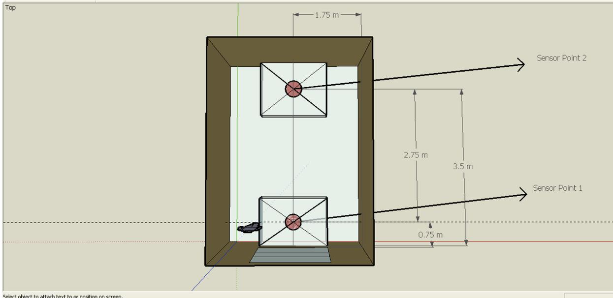
Figure 3-2. Top view the office building with the two sensor points positioned on two office desks.
