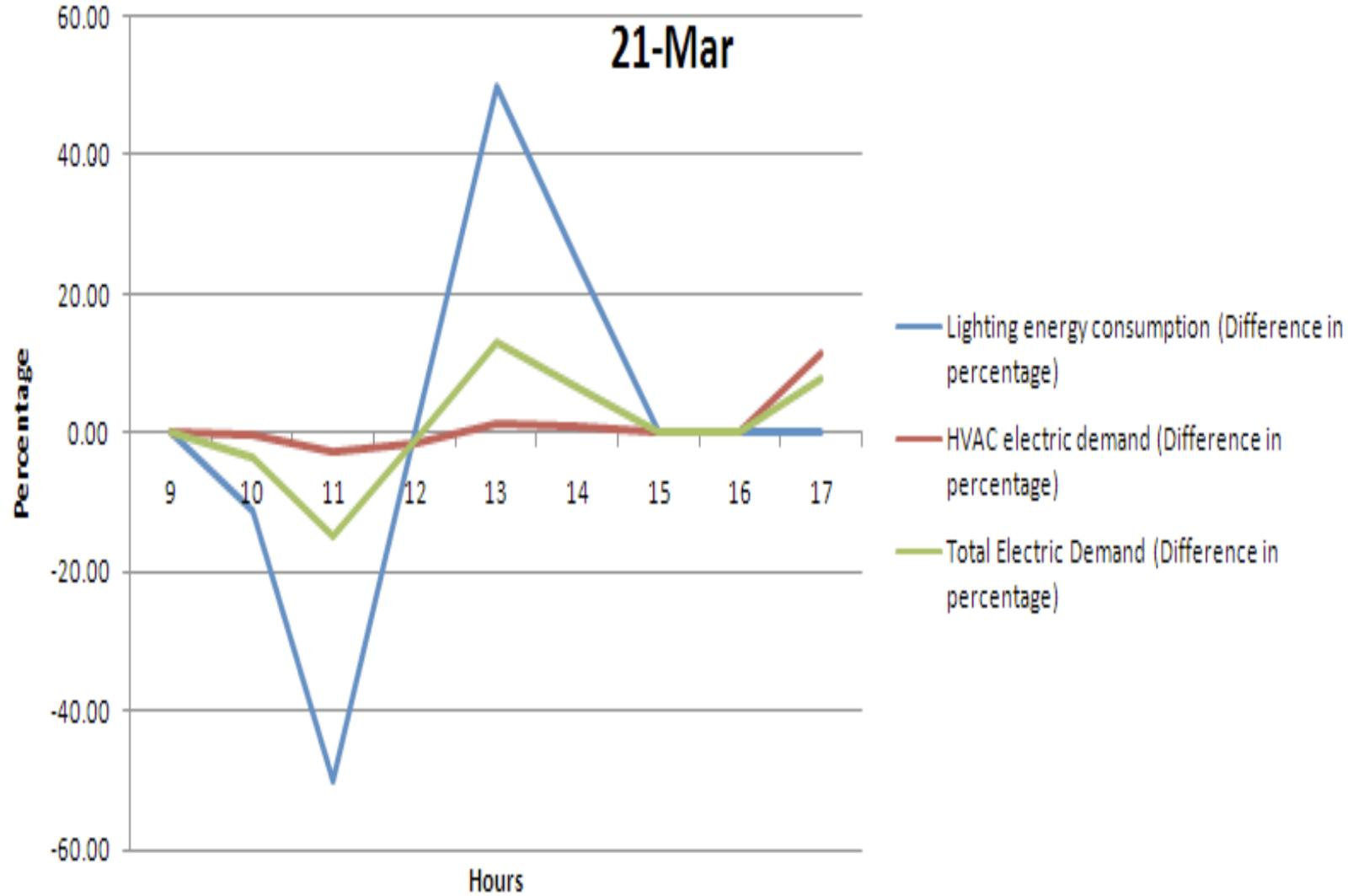
Figure 4-1. Energy consumption differences between split-controlled blinds and conventional blinds for March 21st
