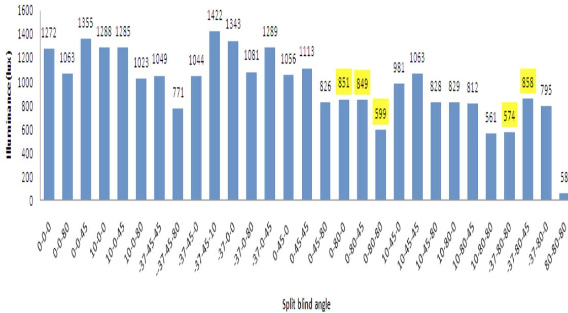
Figure 4-10. Illuminance values for all the split blind angles, at the first sensor point for January 1 at 8 a.m.
