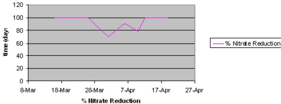
Figure 6-4. Performance of attached growth bioreactor (% nitrate reduction vs. time)
