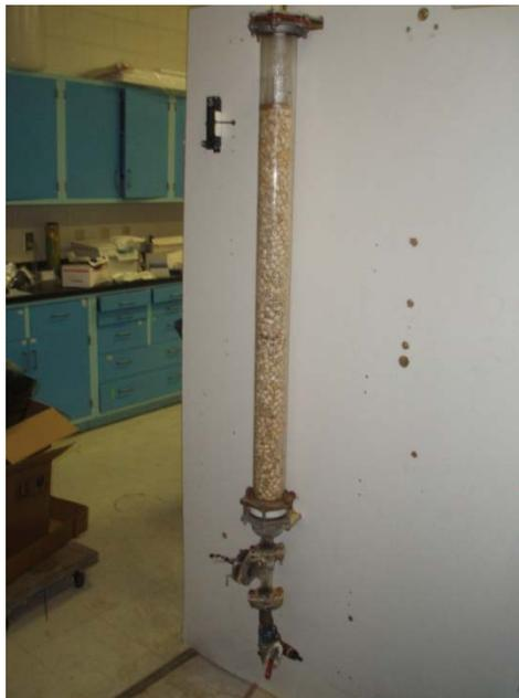
Figure 5-1. Packed column for aeration experiments
