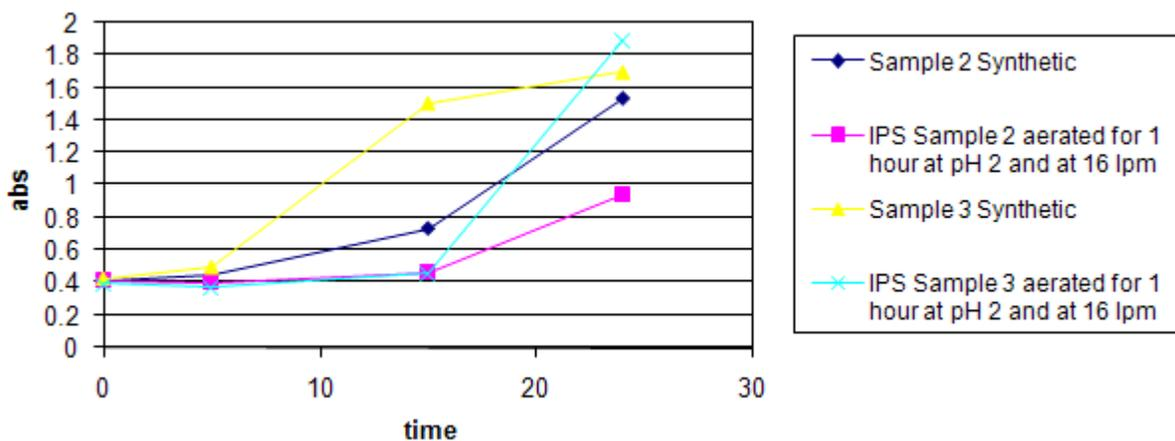
Figure 3-12. Absorbance results for aeration IPS samples 2 and 3
