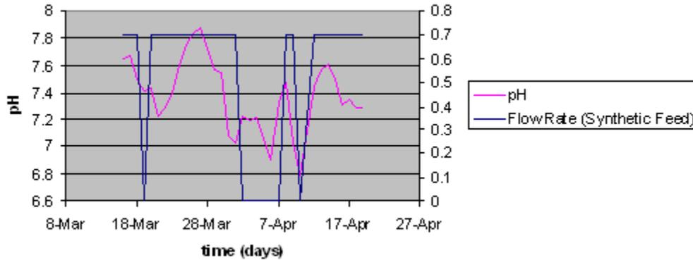
Figure 6-3. Performance of attached growth bioreactor (pH vs. time)
