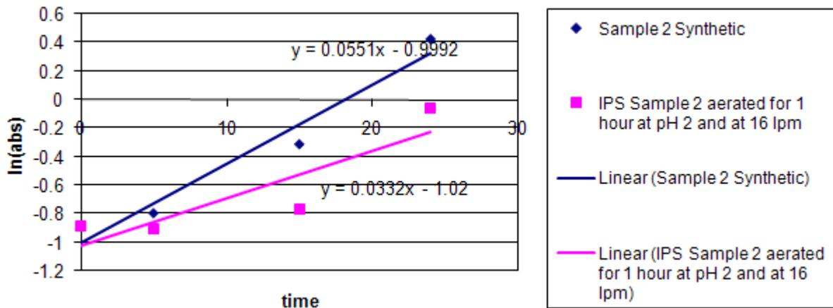
Figure 3-13. BI for aeration IPS samples 2
