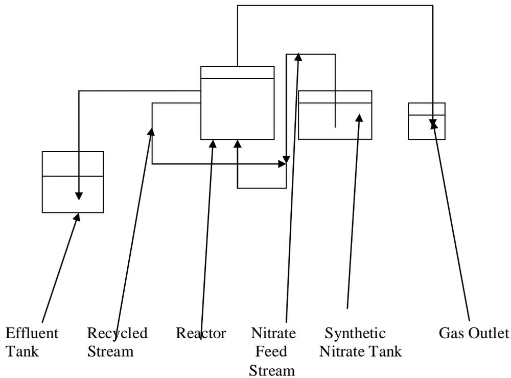
Figure 6-2. Block diagram of the attached growth reactor assembly
