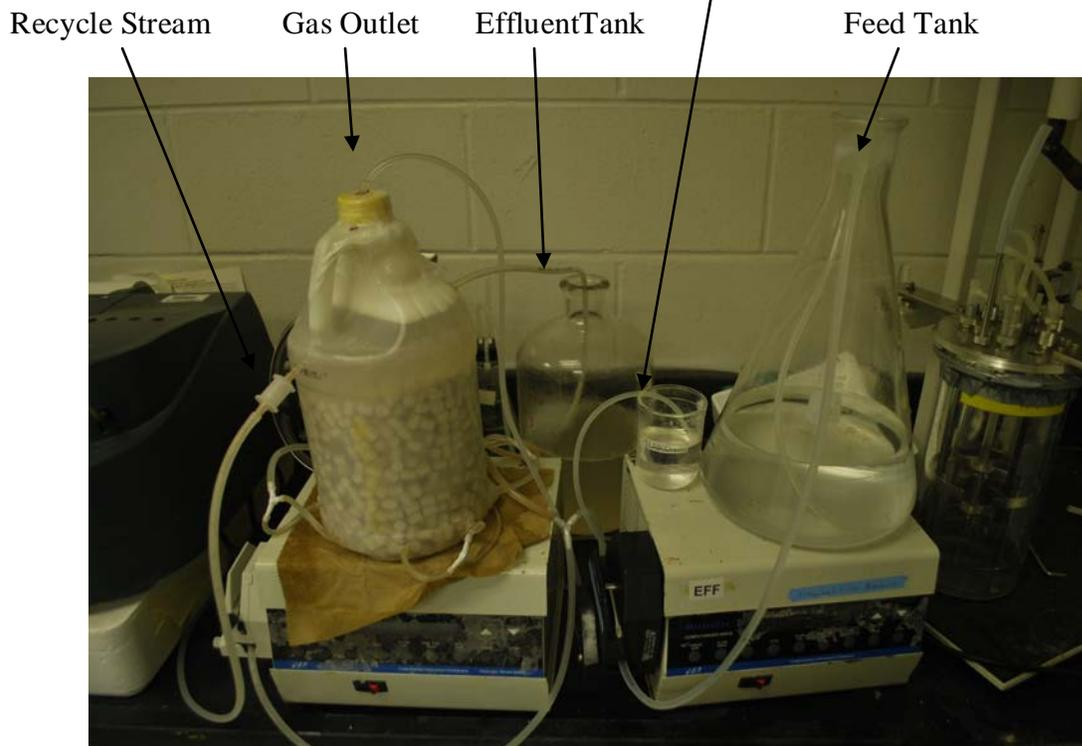
Figure 6-1. Experiment setup for attached growth reactor
