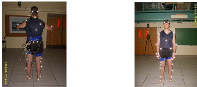
Figure 3-5. Placement of the retro reflective markers and the wireless EMG transmitter
