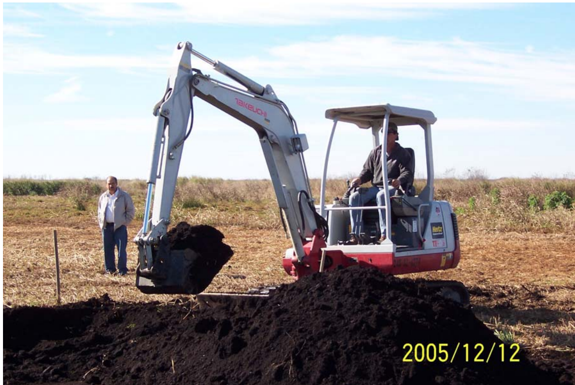
Figure 4-2. Soil mixed in a 13 ft x 13 ft plot at site ZSS0750 by a trackhoe prior to collection and transport to the greenhouses at the Department of Soil and Water Science, University of Florida, Gainesville.
