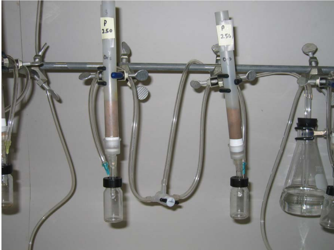
Figure 2-1. Columns containing 20g of soil were kept under 20 cm of suction utilizing Erlenmeyer flasks to ensure unsaturated flow of leachate, which was collected in glass vials.
