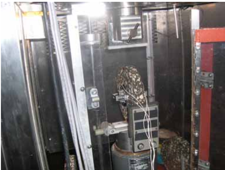
Figure 3-6. Superpave Indirect Tensile Test (IDT)
