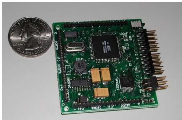
Figure 4-2. Image of the sensor processor module
