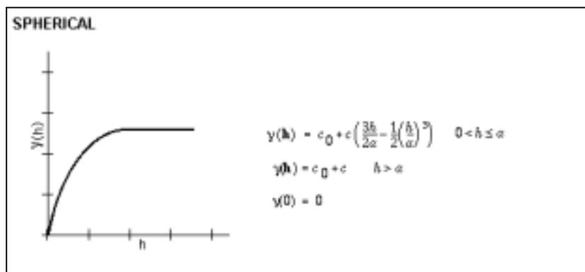
Figure 3.1. The spherical semivariogram equation and functional form.
