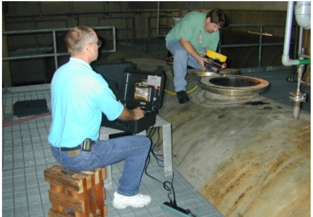
Mike Lane, an electrical engineering technician, lowers Video Ray Pro into a fuel storage tank as Steve Van Meter, a hazardous duty robotics specialist, prepares to operate the robot.
