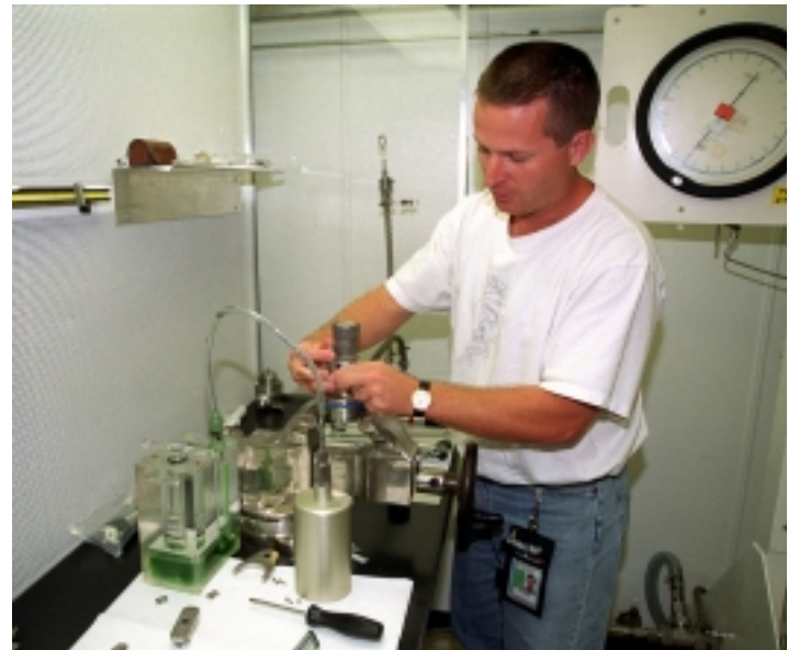
United Space Alliance technician Elliott Clement, above, performs ground half coupling leak checks at the Hypergolic Maintenance Facility. At left, Ralph Gentner and Rusty Allen, right, prepare to weld a replacement check valve in Atlantis' OMS pod. Below, Walter Schmitz, HMF engineering lead, inspects a forward module.
