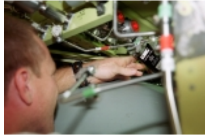
Above, technician Rusty Allen sets up equipment to weld a replacement check valve in Atlantis' right hand OMS pod. At left, United Space Alliance technician Walter Harris rebuilds a hypergolic ground half coupling in the quick disconnect lab. Below, one of Columbia's OMS pods waits in storage while Atlantis' OMS pod is repaired in the HMF's east test cell.
