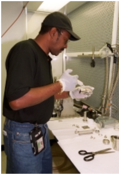
Above, technician Rusty Allen sets up equipment to weld a replacement check valve in Atlantis' right hand OMS pod. At left, United Space Alliance technician Walter Harris rebuilds a hypergolic ground half coupling in the quick disconnect lab. Below, one of Columbia's OMS pods waits in storage while Atlantis' OMS pod is repaired in the HMF's east test cell.
