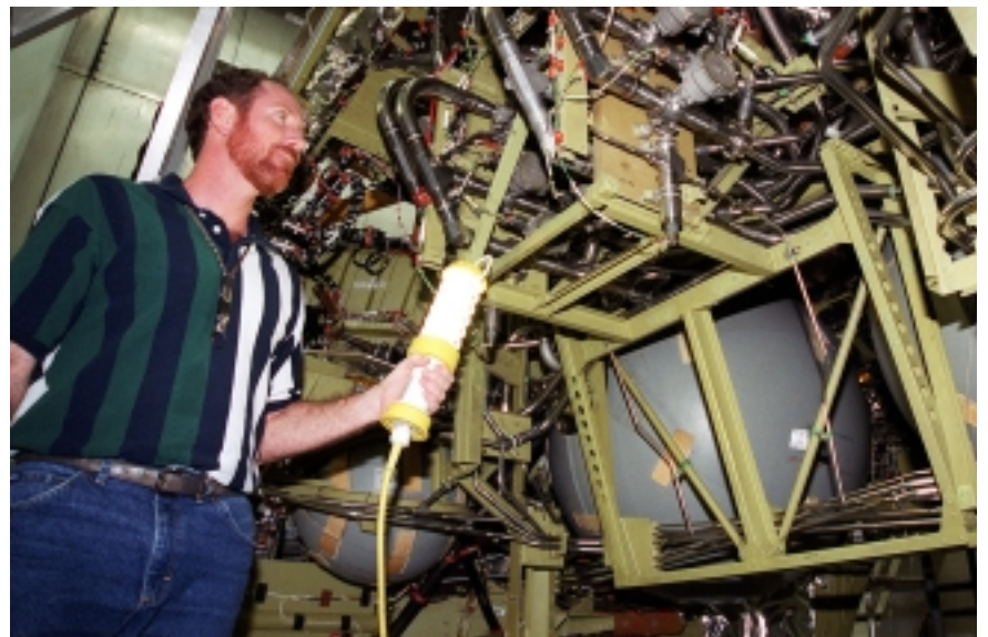
United Space Alliance technician Elliott Clement, above, performs ground half coupling leak checks at the Hypergolic Maintenance Facility. At left, Ralph Gentner and Rusty Allen, right, prepare to weld a replacement check valve in Atlantis' OMS pod. Below, Walter Schmitz, HMF engineering lead, inspects a forward module.
