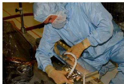
John O'Brien checks a diode box for the Rigid Array Carrier.
