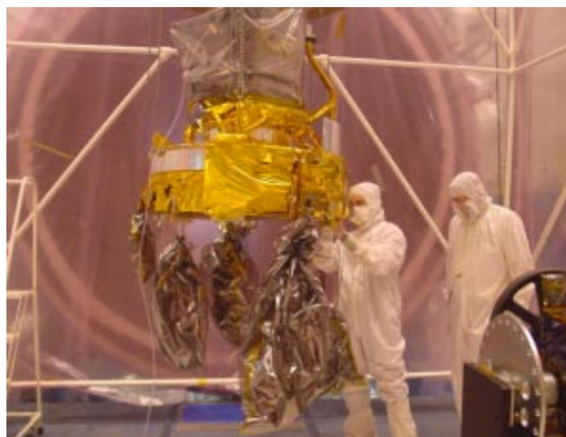
Workers perform a thermal vacuum test prep of the QuikTOMS satellite at Vandenberg Air Force Base, Calif.
