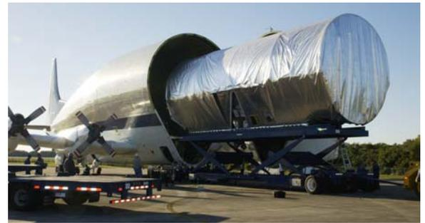
The Long Spacer, the second piece of the Starboard 6 Integrated Truss Segment, rolls out of the Super Guppy.
