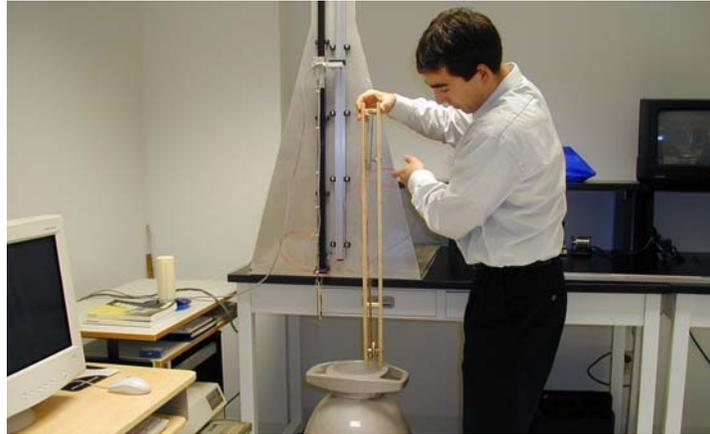
The Cryo-Tracker™ liquid level and temperature sensor for cryogenic fluids undergoes flexibility testing in liquid nitrogen at Sierra Lobo.
