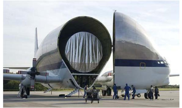
The Integrated Equipment Assembly is offloaded from NASA's Super Guppy cargo airplane following its arrival at the Shuttle Landing Facility. The customized four-engine aircraft has a 24-foot-diameter fuselage and a foldaway nose enabling it to load and transport oversize cargo.
