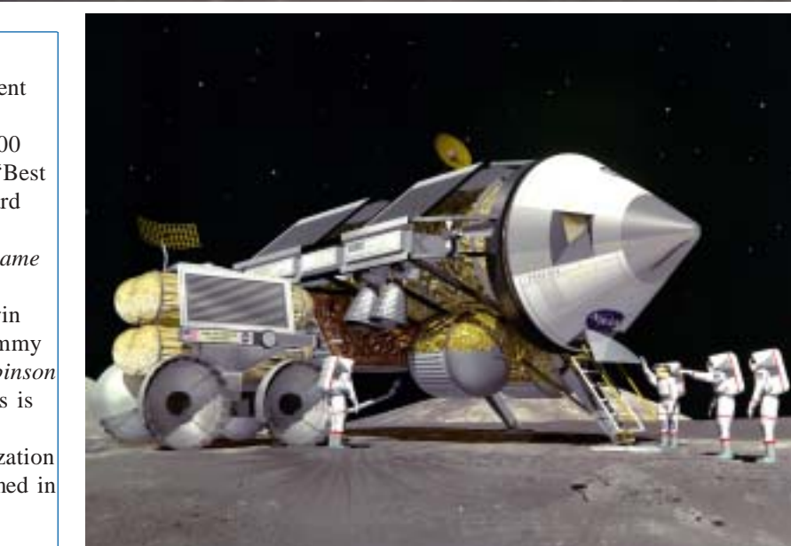
A LUNAR CREW refills the propellant tanks on its spacecraft with oxygen produced on the Moon in this artist's concept. This would allow the astronauts to return directly to Earth, reentering the atmosphere in the conical crew module and touching down at a prepared landing site.
