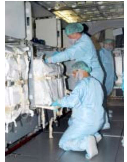
ABOVE, technicians begin moving resupply stowage bags into the Italian-built Raffaello. The bags will be placed in containers known as resupply stowage racks.
