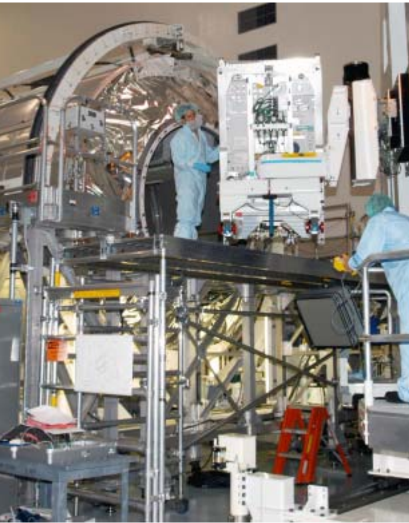
AT LEFT, in the Space Station Processing Facility, the Rack Insertion Device moves the Human Research Facility-2 science rack toward Raffaello (at left).
