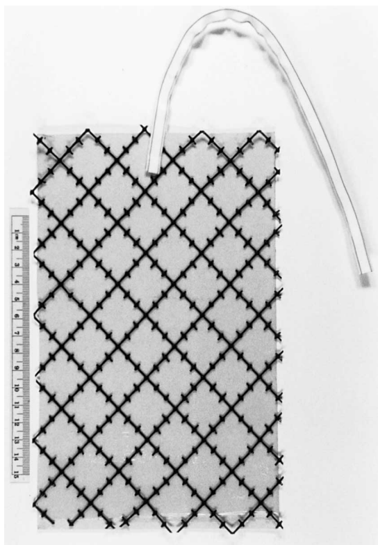
Fig. 1. Sticky trap (23 × 14 cm) for fruit flies constructed with yellow or green fruit fly adhesive paper covered with plastic mesh (2.2 × 2.2 cm mesh).
