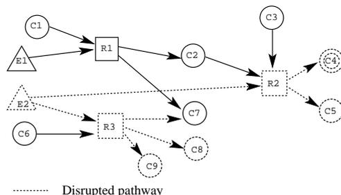
Figure 1. A graph constructed for a hypothetical metabolic network with three reactions  $R_1$ ,  $R_2$ , and  $R_3$ , three enzymes  $E_1$ ,  $E_2$ , and  $E_3$ , and nine compounds  $C_1, \dots, C_9$ . Circles, rectangles, and triangles denote compounds, reactions, and enzymes respectively. Here,  $C_4$  (shown by double circle) is the target compound. Dotted lines indicate the subgraph removed due to inhibition of enzyme  $E_2$ .
