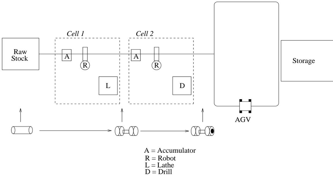
Figure 3: Manufacturing line with two robots and two machines..
