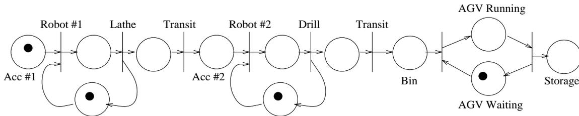
Figure 4: Petri net model for manufacturing line.
