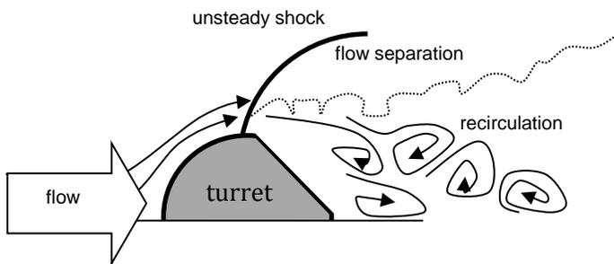
Figure 1. Flow schematic around aero-optical aircraft turret at transonic speeds.
