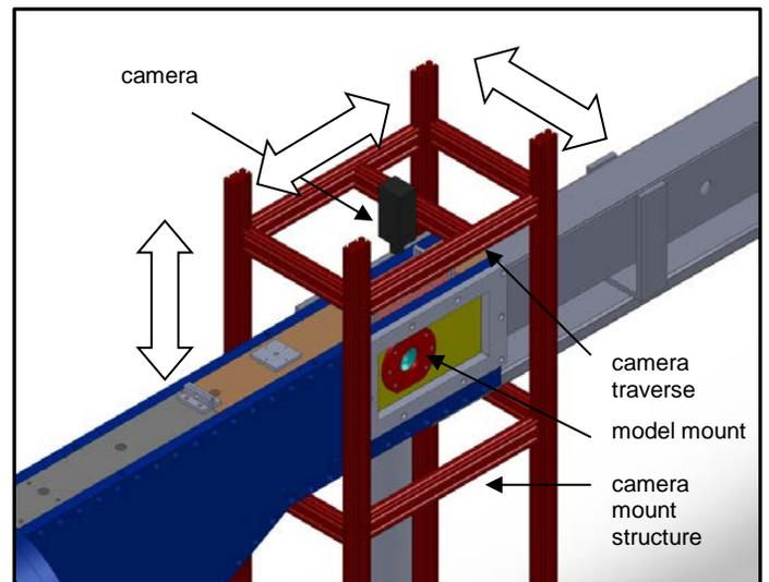
Figure 11: Camera mount structure.
