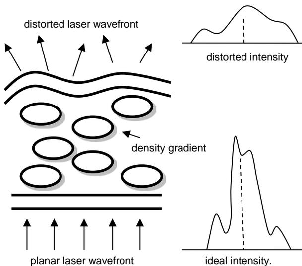
**Figure 3.** Schematic (not to scale) of aero-optic effect on laser intensity [1][3].
