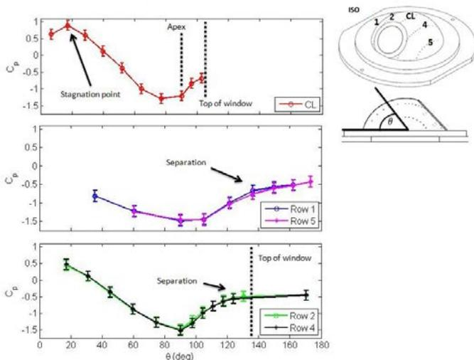
**Figure 6.** Model steady pressure measurements with respect to  $\theta$  for (a) the centerline, (b) rows 1 and 5, (c) rows 2 and 4. These results were obtained by Benjamin George at the University of Florida transonic wind tunnel facility. Notice the location of the stagnation point, separation, and high pressure region.
