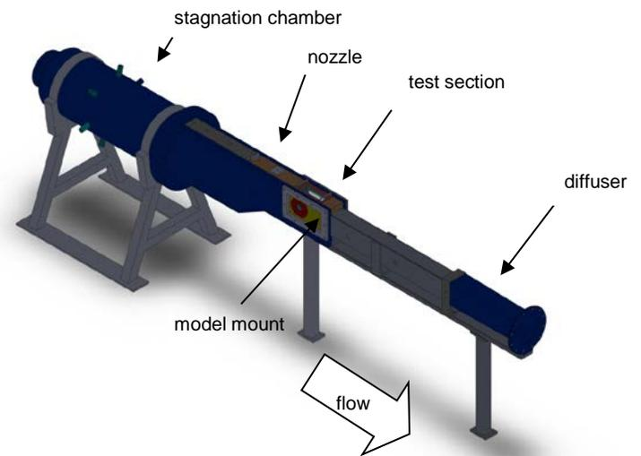
**Figure 8.** University of Florida transonic wind tunnel.
