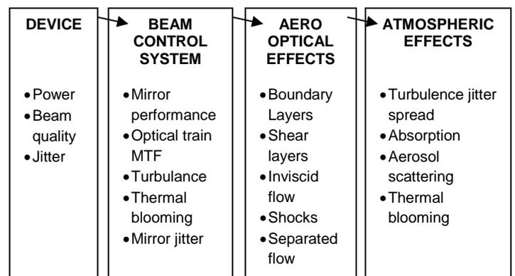
Figure 2. Sources of laser degradation [1].
