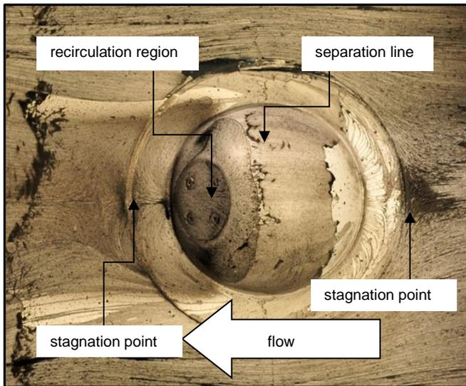
**Figure 5.** Oil flow visualization results turret courtesy of Benjamin George at the University of Florida transonic wind tunnel facility. Notice the location of the recirculation region and stagnation points.
