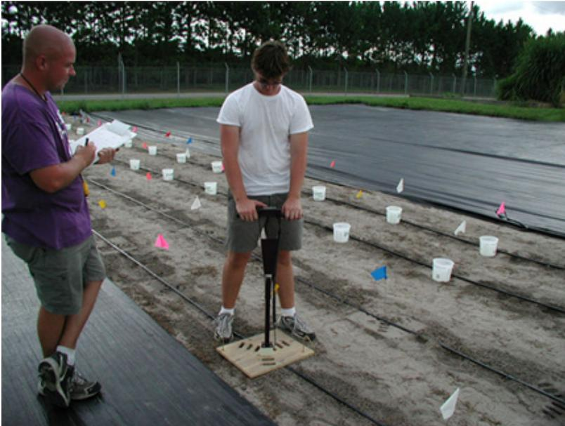
*Figure 2. Taking soil moisture measurements with the TDR probe during a test.*
