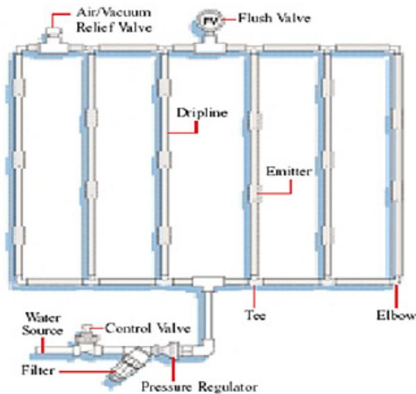
Figure 1. Typical microirrigation system layout.
