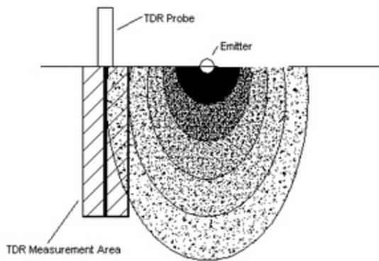
*Figure 5. Wetting front of the drip emitter compared to the measurement area of the TDR probe at the 15 cm distance.*
