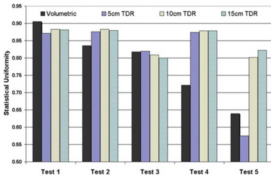
Figure 6. Statistical uniformity calculated by equation 4 for volumetric measurements and soil moisture measurements at three distances from the emitter.
