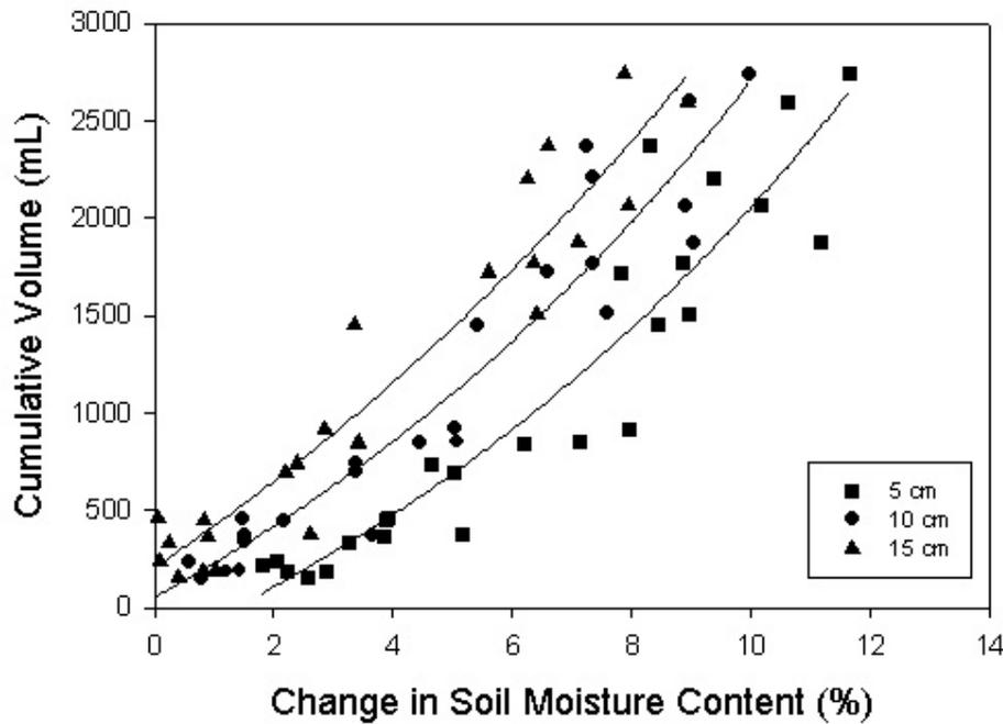
Figure 3. Relationship between volume emitted and the change in soil moisture at 3 distances from the emitter.
