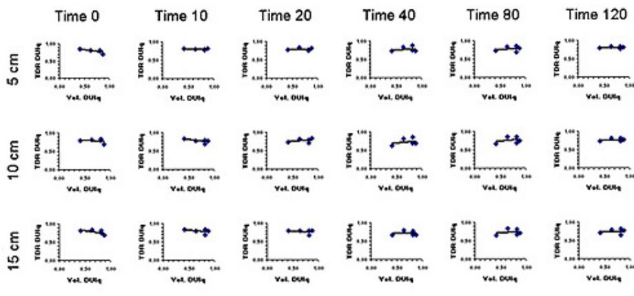
Figure 4. Comparison of low-quarter distribution uniformity calculated by soil moisture content (TDR  $DU_{1q}$ ) and volumetrically (Vol.  $DU_{1q}$ ).
