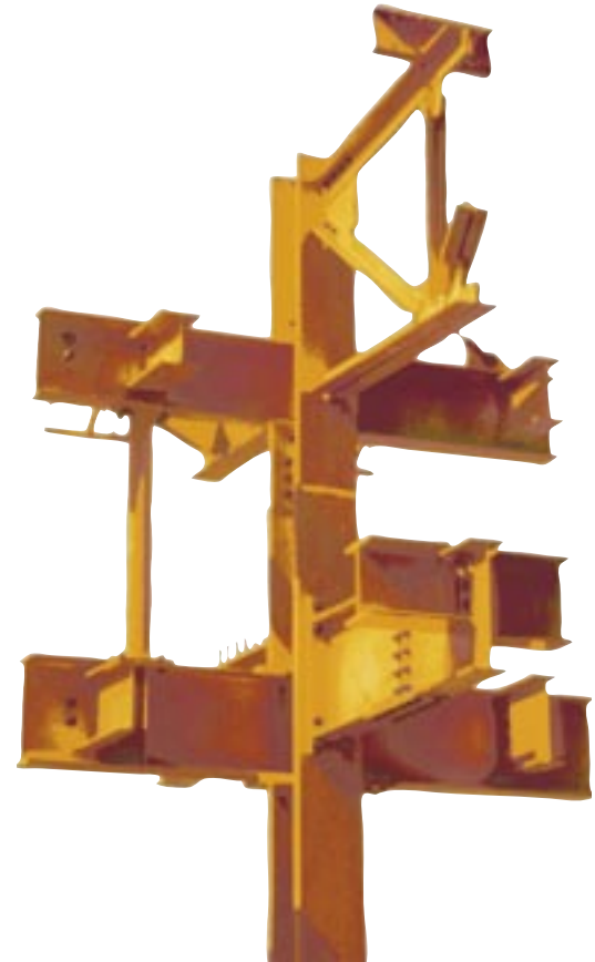
Steel teaching sculpture, created by Dr. Duane Ellifritt, University of Florida. Now in use by Civil Engineering departments across the nation.
