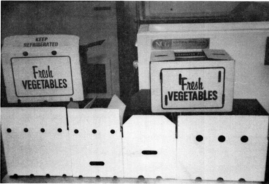
Figure 7. Several currently used and experimental containers with vents of various sizes, shapes, and locations.
