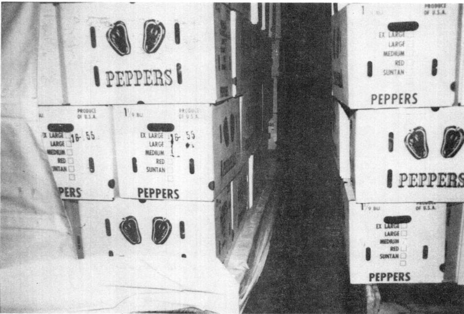
Figure 6. Plastic used to seal the pallet opening in the row of pallets on the left.
