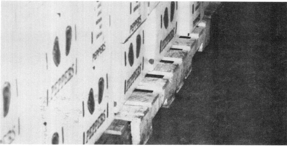
Figure 5. Opening in tops of pallets and misalignment of pallets forming forced-air cooling tunnel.
