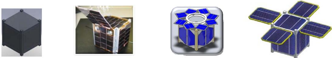
(a) baseline design    (b) CUTE-1 fold-out [7]    (c) circumferentially actuated    (d) Four-panel fold-out [4]
