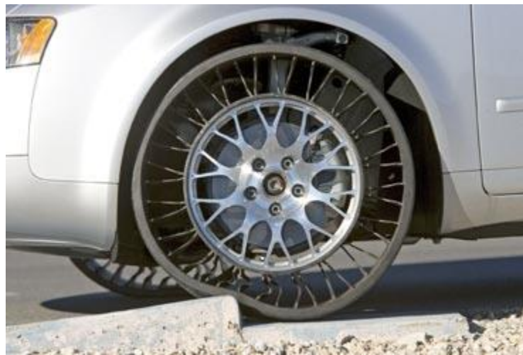
Fig. 4. The Michelin Tweel Airless Tire [18].
