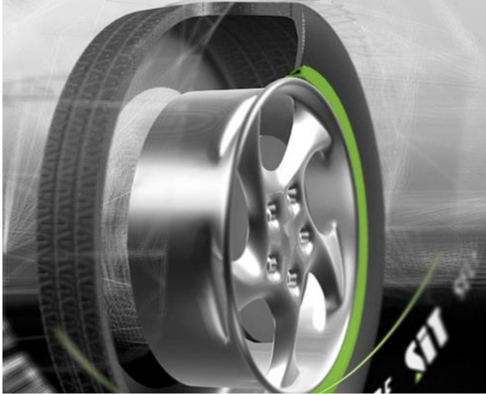
Fig. 2. Coda Development's Self-Inflating Tire [16].
