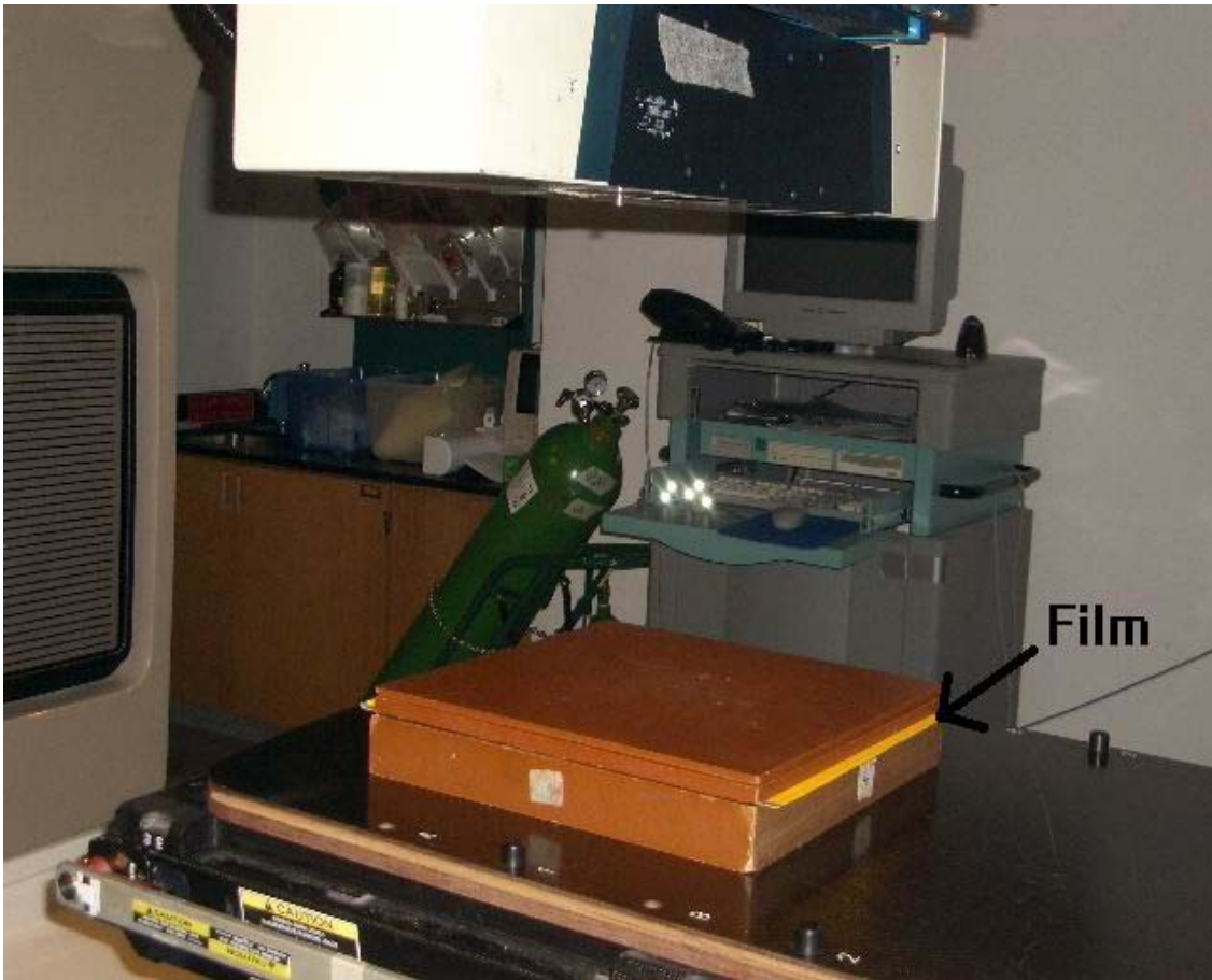
Figure 2-1. Basic setup for film measurements. Kodak radiographic film is sandwiched between two slabs of solid water.
