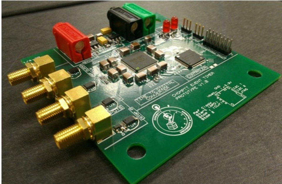
Figure 2-6. Event Timer electronics board of OPTI 1. Photo courtesy of author.
