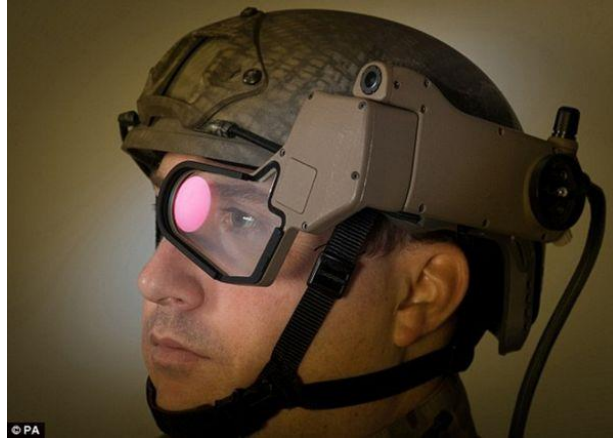
Figure 2-5. Military Augmented Reality headset (Photo Courtesy: Meghan Young, Baesystems, and device (Meghan 2014)).
