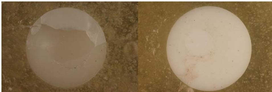
Figure 3-9. Failure of IPS Empress ceramic (IP) which had been etched before bonding (left). No such failures occurred in any of the Cercon Zirconia specimens (CZ), independent of surface treatment (right).
