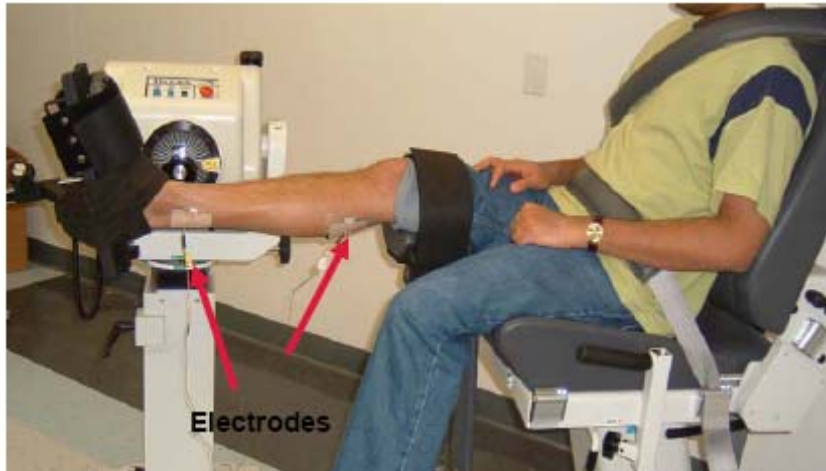
Figure 3-3. Experimental set-up on a Biodex System 3 Dynamometer.
