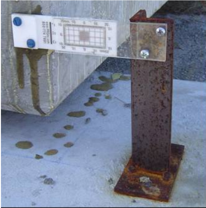
Figure 38. Displacement gage attachment bracket
