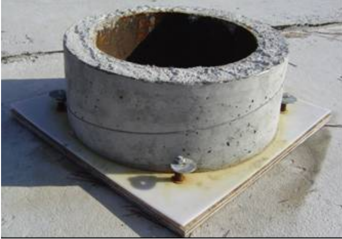
Figure 41. Typical restrained ring specimen
