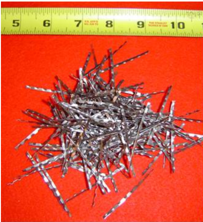
Figure 31. Steel fibers used in BND and STL toppings
