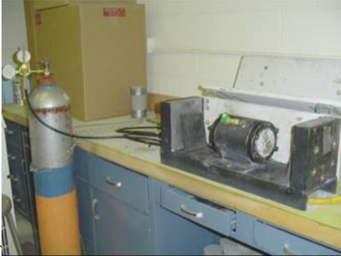
Figure 28. Pressure tension testing equipment (Li 2004)
