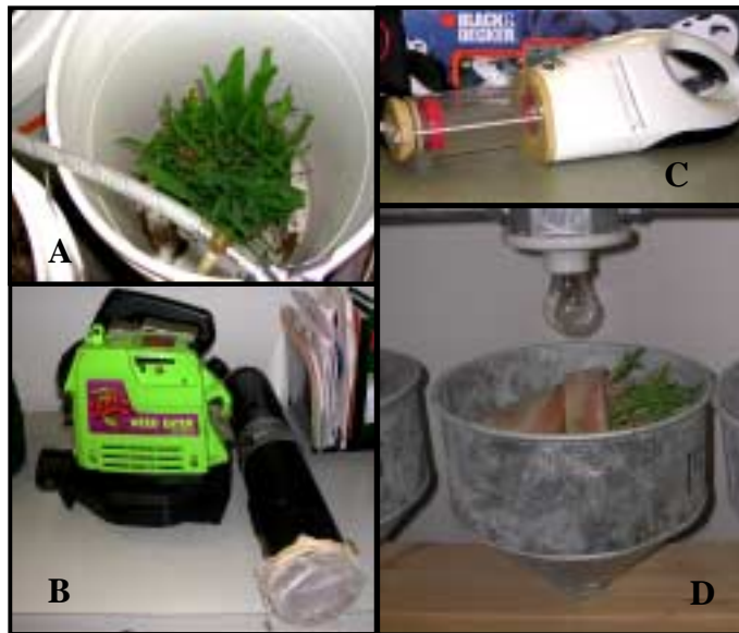
Figure 2-2. Equipment used to recover Blissus insularis from test plants. A. Flotation method. B. Large blower/vacuum. C. Hand-held vacuum. D. Berlese funnel.
