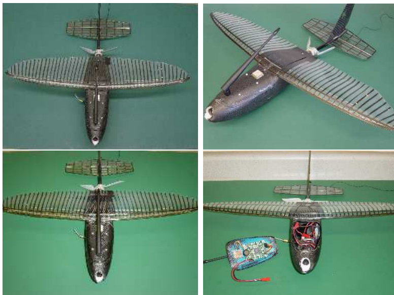
Figure 5-1: MAV Prototype for Vision-Based Control
