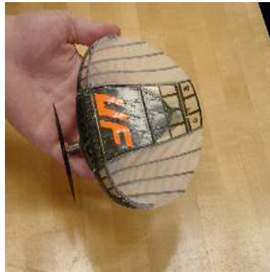
Figure 1–1: Flexible Wing Concept on a 6 in MAV
