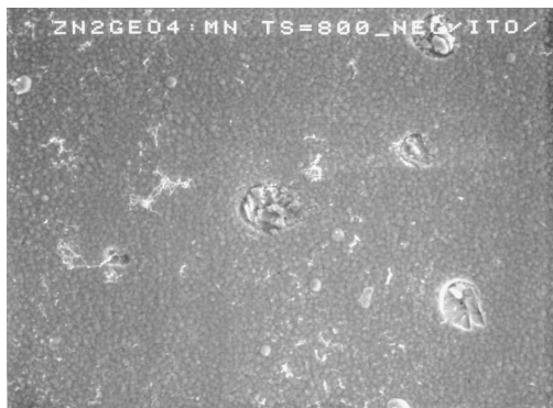
Figure 4-13 SEM image of \text{Zn}_2\text{GeO}_4\text{:Mn} deposited at substrate temperature 800^\circ\text{C} on glass/ITO/ATO substrate (UF-ATO-1)
