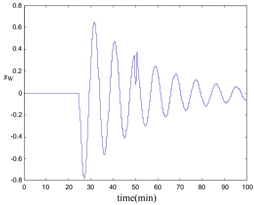
Figure 6.4 Opening of the Water Valve
