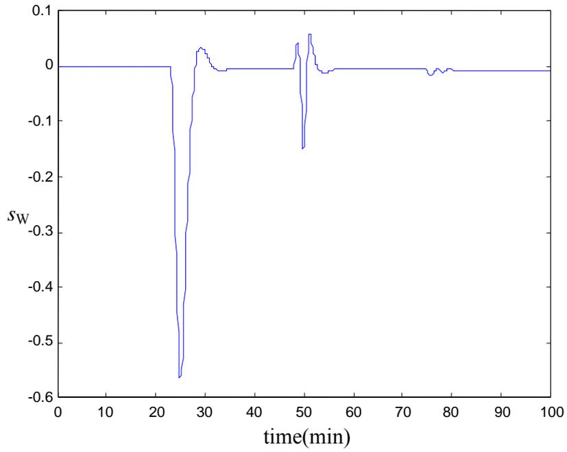
Figure 6.16 Opening of Valve of Water
