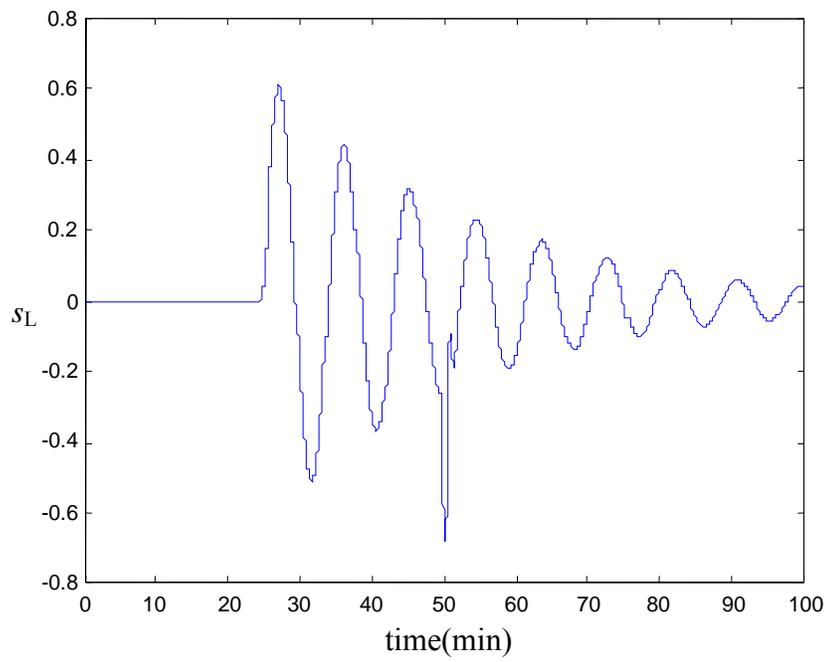
Figure 6.5 Opening of the Oil Valve
