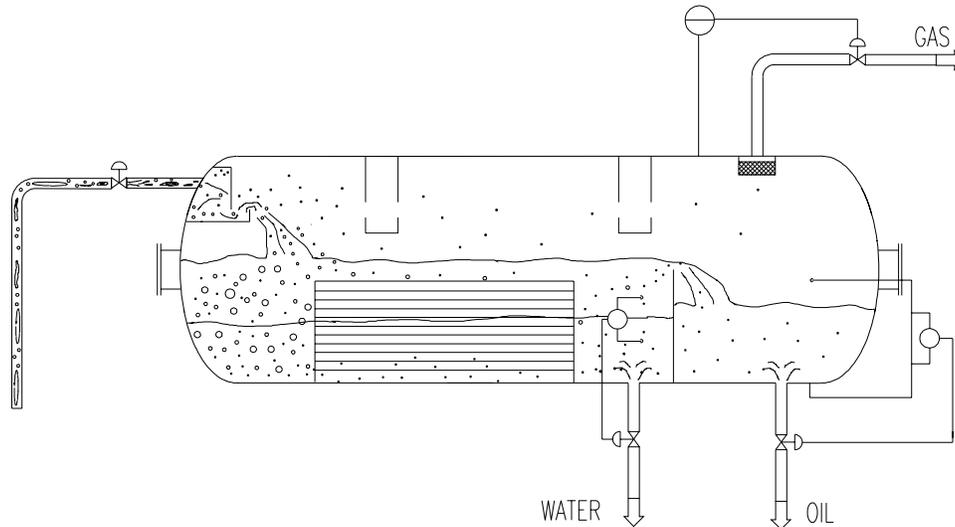
Figure 5.1 Oil-Water-Gas Separator
