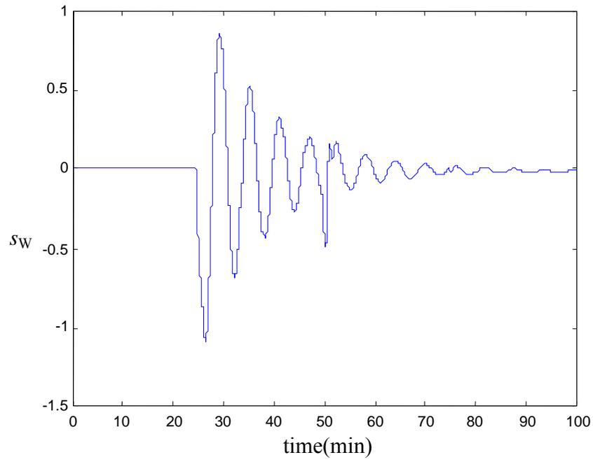
Figure 6.10 Opening of Water Valve
