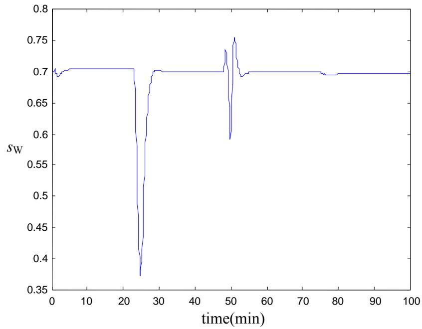
Figure 7.10 Opening of Water Valve
