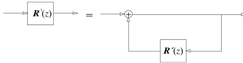
Figure 4.2 Inversion of  $\mathbf{R}$  in Simulink
