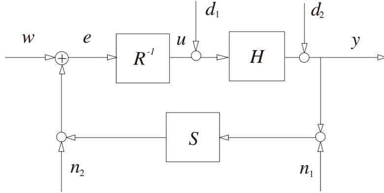
Figure D.1 Closed-loop system with external disturbance and noise signals
