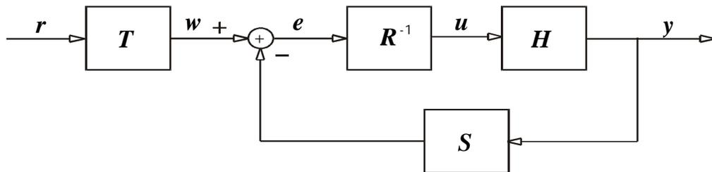
Figure 4.1 Closed-loop System
