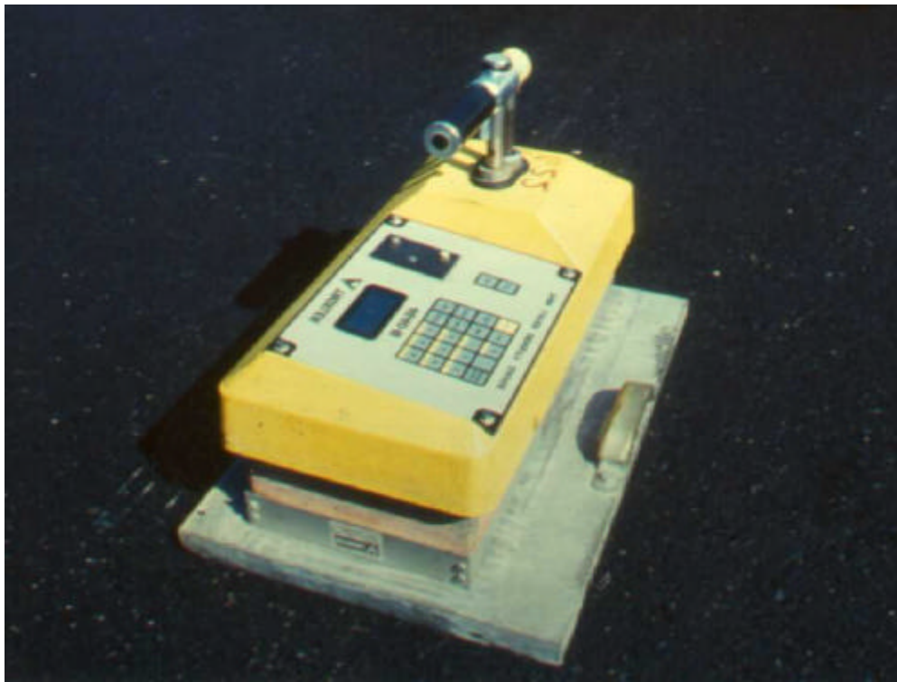
Figure 4-1. Nuclear Gauge Instrument (Obtained photo from Joint AASHTO-FHWA Industry Training Committee on Asphalt)
