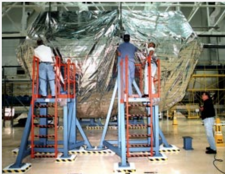
Workers adjust the connection of the port-side P3 truss on its workstand in the Operations and Checkout Building on Nov. 17. The truss, a segment of the International Space Station (ISS), is scheduled to be launched on mission STS-115 in 2002 aboard the Space Shuttle Atlantis.
