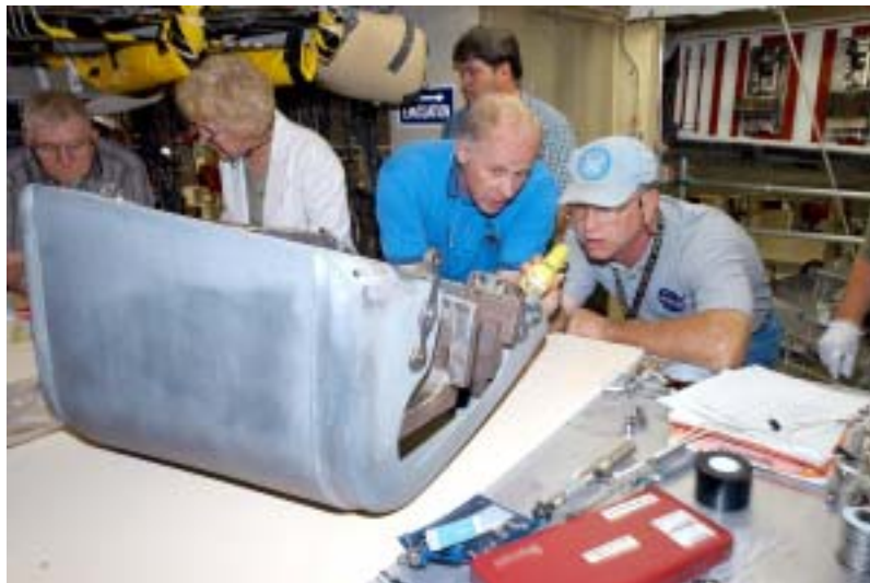
IN THE ORBITER PROCESSING FACILITY, Danny Wyatt, NASA Quality Assurance specialist, and John Legere (right), NASA Quality Assurance specialist, examine the first Reinforced Carbon-Carbon panel to be installed on the left wing leading edge on Discovery.
