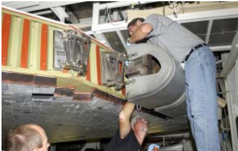
UNITED SPACE ALLIANCE employee Mike Hyatt (above) finishes installing a Reinforced Carbon Carbon panel to the leading edge of the wing of the orbiter Atlantis.
