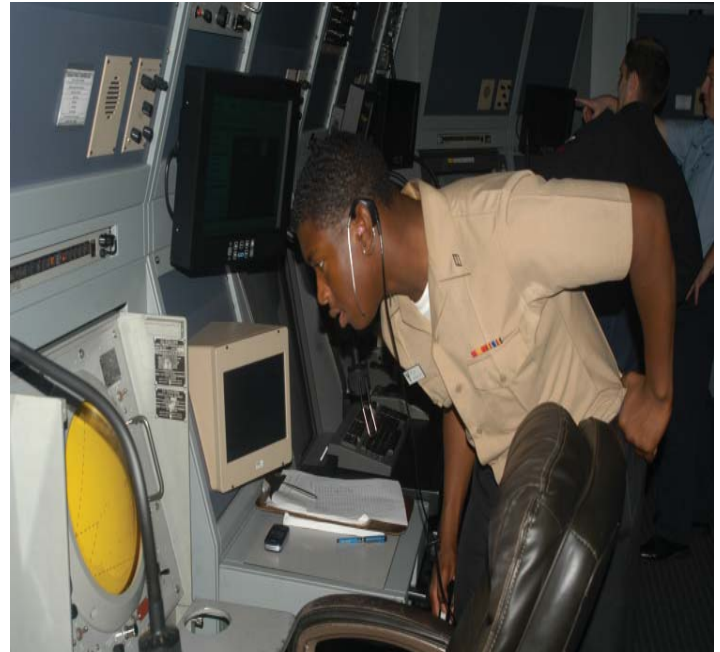
Air traffic controller (ATC) Airman Jermaine Roby responds to a radio call from an inbound pilot. Roby guides the pilot in using precision approach radar. ATCs executing precision approaches ensure pilots are on the proper glide path and heading while landing. U.S. Navy photo by Lt. j.g. Daniel Ammons-Moreno.
