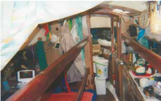
'Not pretty, but it works' Above: Shoulder- and waist-high rails prevent injury below in heavy weather Top right: The former dining table is now a permanent berth
