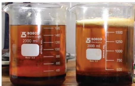
**Biodiesel produced in a lab: top layer is biodiesel, bottom layer is glycerol**
