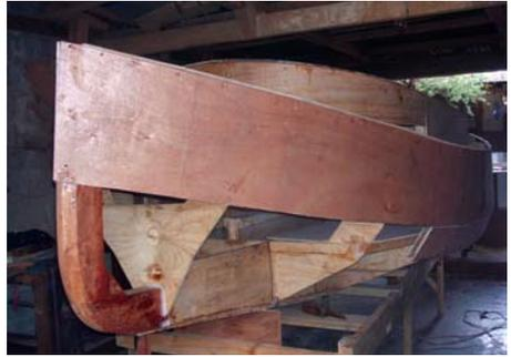
**The first topsides plank, the cabin sides and part of the first bilge planks are fastened**
