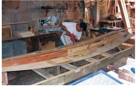
**The bottom plank with the centerboard trunk stiffeners in place being screwed to the building platform by David Ramirez**
