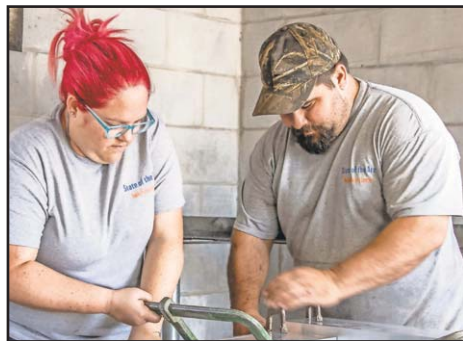
Farren and Charlie square up the corner of an aluminum gate for welding.
