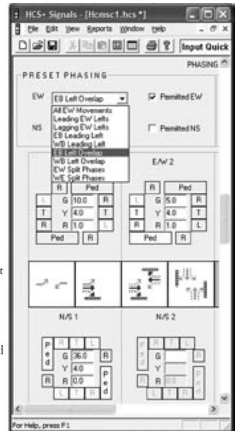
**I-Value:** The ability to import upstream signal data to get the volume-to-capacity ratios for determining the I-Value for each approach has been added. The volume-weighted average of the contributing movement is used to select the appropriate I-Value from HCM 2000 Exhibit 15-7.
