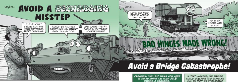
Mechanics, figuring out why a Stryker's batteries aren't charging can be tricky and time consuming. But you might save yourself some trouble by making the W4 cable inside the troop compartment one of your first checks.
