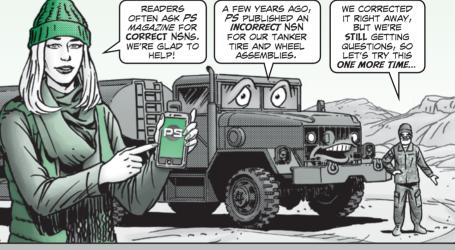
TO ORDER A **REPLACEMENT TIRE AND** WHEEL ASSEMBLY FOR THE M967A1 AND M969A1/A2 FUEL TANKER, USE NGN 2530-01-506-4125. THAT BRINGS A NEW 22.5-IN TUBELESS TIRE WITH A ONE-PIECE WHEEL (WHICH IS
