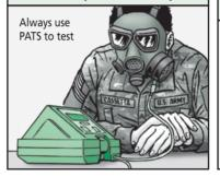
If a small mask is too big to create a good seal, readjust and tighten the head harness, then test with PATS again. Sometimes that's enough to do the trick. If it still flunks, make sure the head harness snaps back when stretched. Replace it if necessary.
