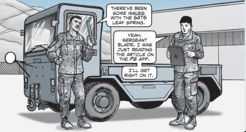
Mechanics, the leaf spring assemblies on the standard aircraft towing system (SATS), NSN 1740-01-575-5662, are experiencing excessive wear that can put the SATS in a non-mission capable status.
