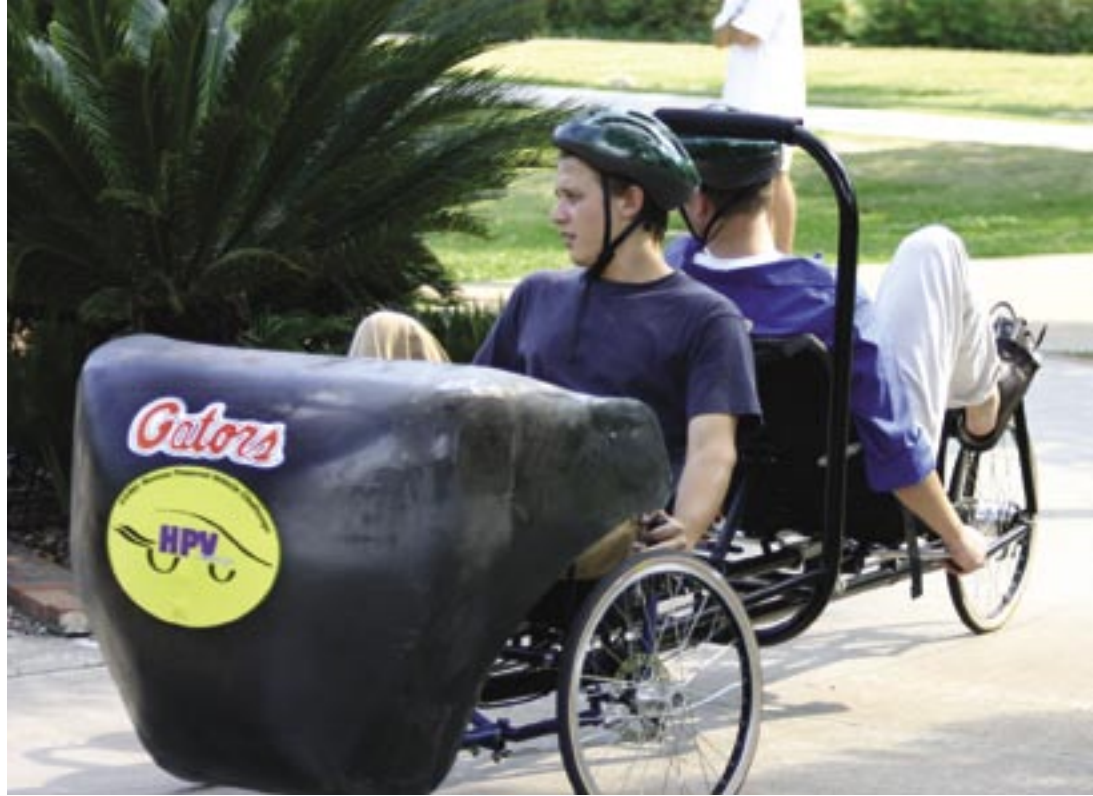
UF Mechanical & Aerospace Engineering students Frank Hartman (rear seat) and Jacob Stoval (front seat) pedal the Instigator II during the safety inspection. Riders must show that the vehicle abides by safety guidelines. Some requirements include making a complete stop in a distance of 20 feet or less from a speed of 15 miles per hour, traveling in a straight line for 100 feet, and negotiating a turn within a 25-foot radius.
